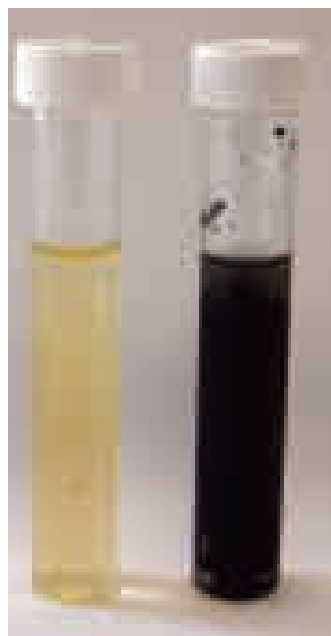
Sig sulphide test for SRB in bottom sample (left unused test; right test showing strong positive)
